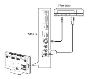
3 Connect an audio cable to the VIDEO IN 1 L and R audio jacks on the side of your TV and to the AUDIO OUT jack on the S-Video device.
